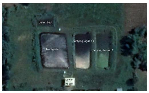
Figure 3. Satellite image of GREG III Farm's Wastewater Treatment Facility (Image generated using Google  $\textit{Earth}^b$ )
