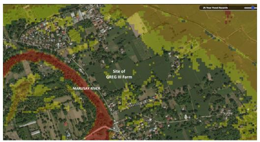
Map 3. Satellite image of GREG III Farm showing areas at risk to flooding (yellow: low; orange: moderate; red: high) (25 year flood hazard; Image generated through Project NOAH<sup>c</sup>)
