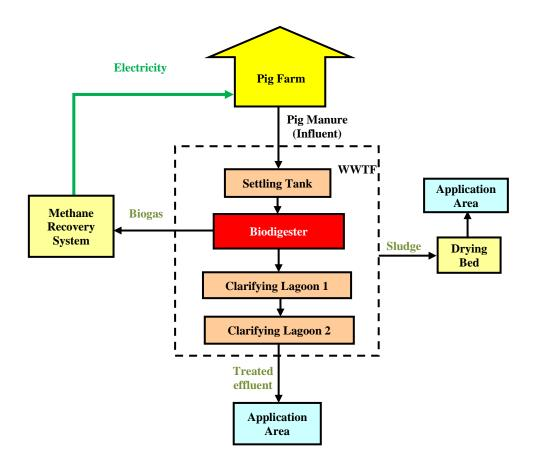
Figure 2. Wastewater treatment process of GREG III Farm
